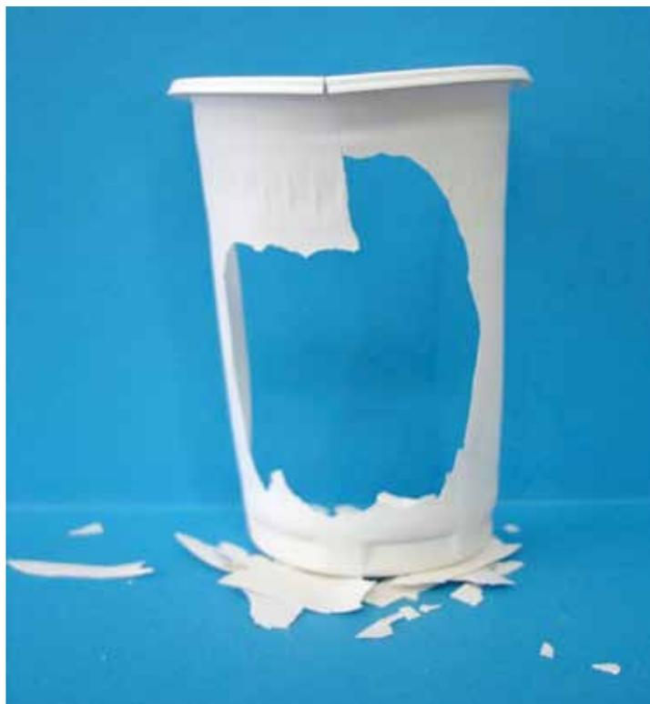
■ A cup containing 2% of Addiflex additive after exposure to ultra violet light for 25 days. ■
