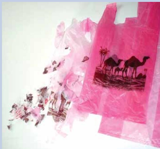
[ A test in industrial compost showed that Addiflex modified polyethylene-film in its unfilled as well as wood-fiber filled version disintegrated during the maturation of industrial compost. ]
